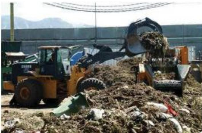
*Bauder appreciates the machine’s ability to handle contaminants mixed with wood fiber.*
