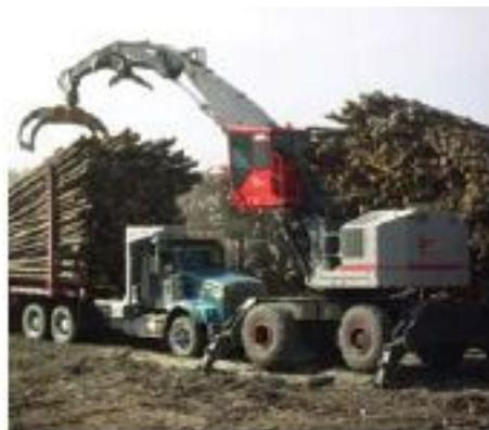
**Machinery Tanguay** Machinery Tanguay manufactures two sizes of wheel knuckle boom loaders. The most popular is the WL350 75,000-lb loader equipped with a Cummins QSB, 6.4 litre engine rated at 225 hp. The smaller WL150 is a 55,000-lb loader, equipped with a 165 hp Isuzu engine.
