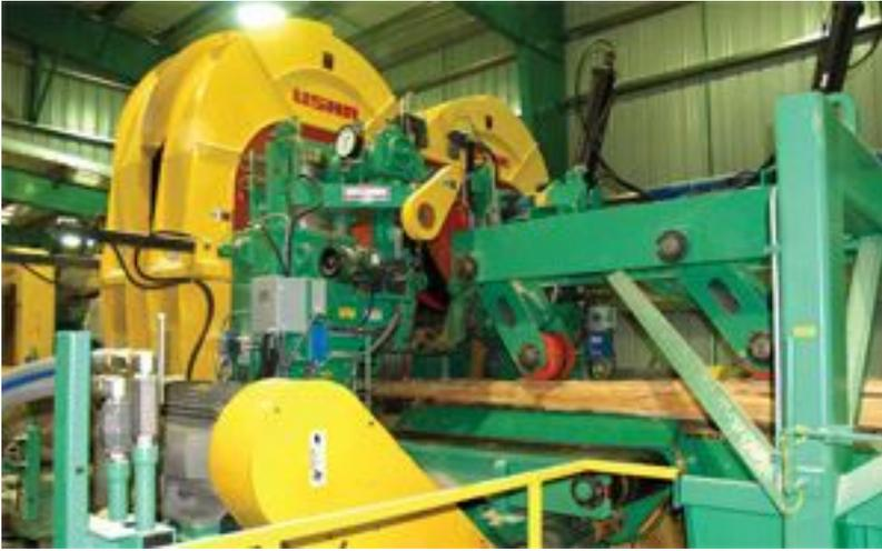
The difference between the Mt Hood mill and Carson mill would be the twin horizontal inline with the double length infeed. “It was pretty much the first time that it had been done,” he adds.
