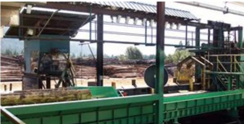
The USNR system also allows WKO to run a large range of log sizes. The system can handle up to 28-inch logs, although WKO doesn’t anticipate running anything larger than 24 inches in diameter. And it can take logs as small as five inches in diameter.
