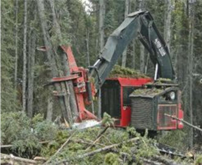
*Oler Bros Contracting does most of its logging on steep ground, which can reach up to a 50 per cent slope, and all of its feller bunchers are tilters. This includes two Timbco 445 EX feller bunchers with Quadco QFH22 heads capable of 360 degree rotation.*
