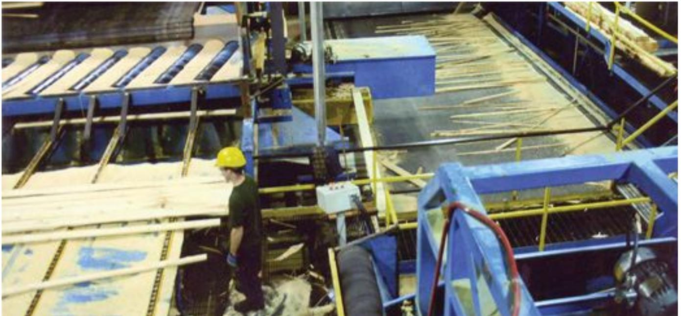
*Logs entering the new saw line (below right). The upgrade meant combining new transfer and conveying equipment with both existing and new mill equipment .*
