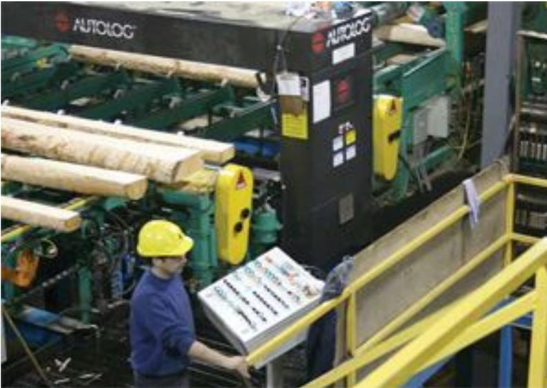
*Logs entering the new saw line (below right). The upgrade meant combining new transfer and conveying equipment with both existing and new mill equipment*
