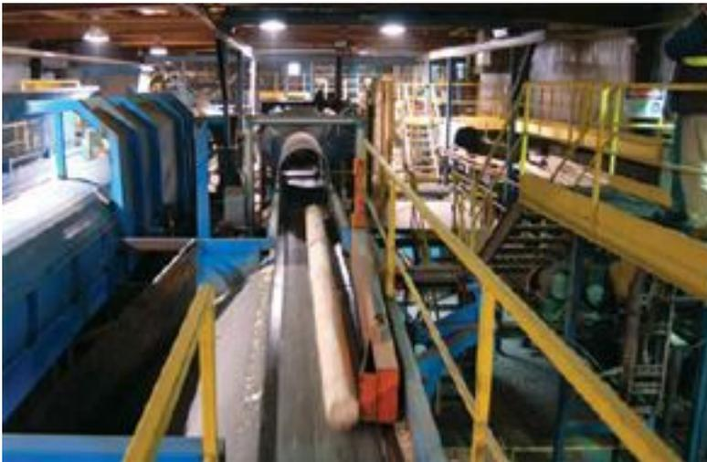
*Among the Comact DDM12's many optimization features are the curve sawing capabilities that promise higher recovery. Thinner blades and the capacity to follow the natural shape of logs will ensure that more fibre is used for lumber and less for waste.*
