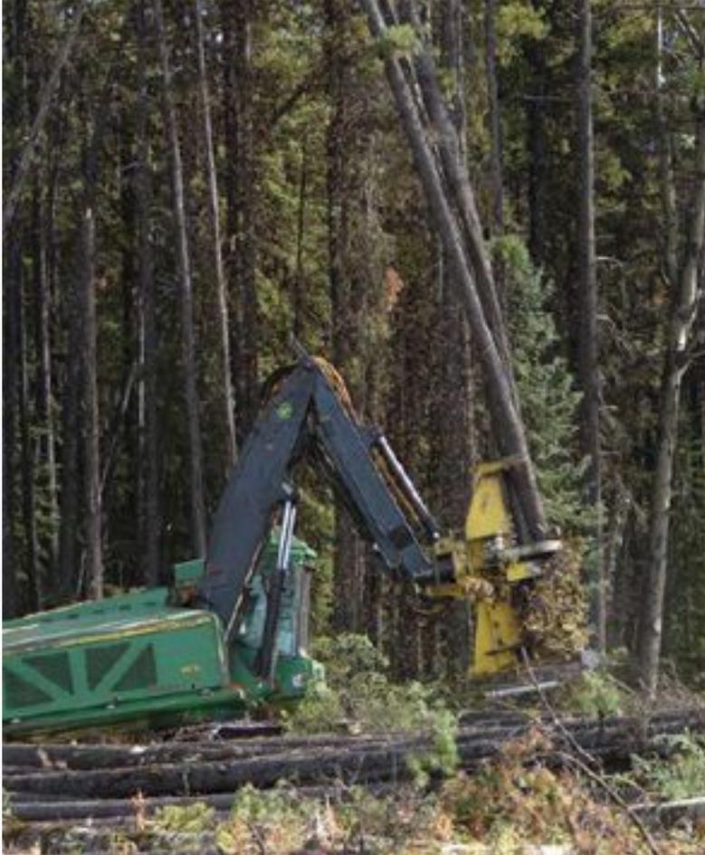
*Westbound Logging has two John Deere 903 feller bunchers with FS22 harvesting heads and Loewen wrist attachments. The attachment gives the heads about 350-degree rotation and is especially handy for careful wood placement, particularly along cutblock boundaries.*
