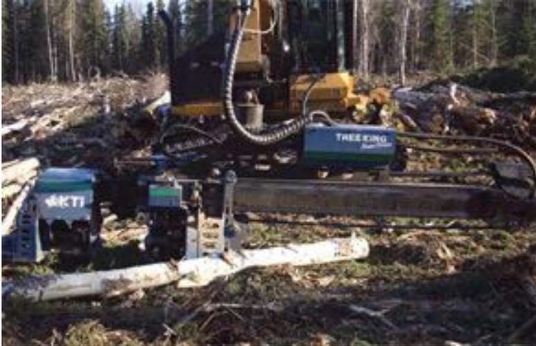
*A unique aspect to the TreeKing processor is that it does not use feed rollers to control and propel logs as they are being delimbed and processed, resulting in less wood damage.*
